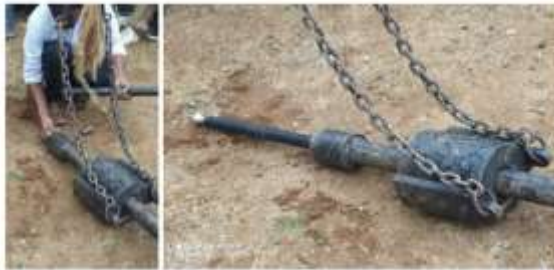
(f) and (g) Fixing guiding rod and dynamic cone to free fall rod and load assembly
