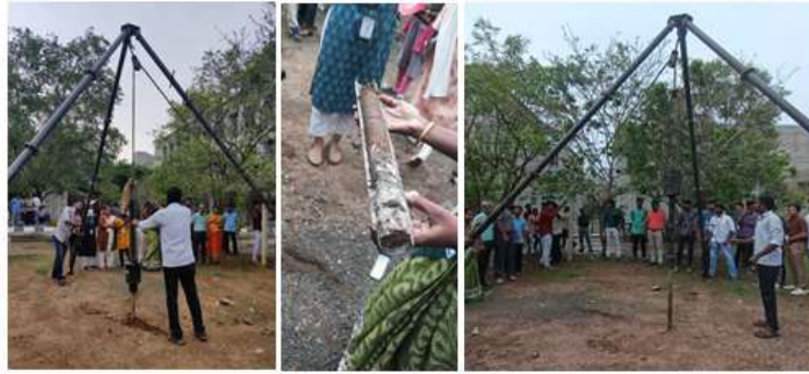
(c) Explaining free fall of 750 mm d) Split spoon sample e) Demo of Standard Penetration Test
