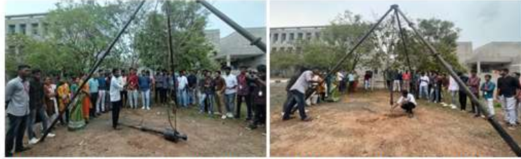
(a) Lifting the load assembly using rope-pulley arrangement b) Verifying the seat drive of split spoon sampler
