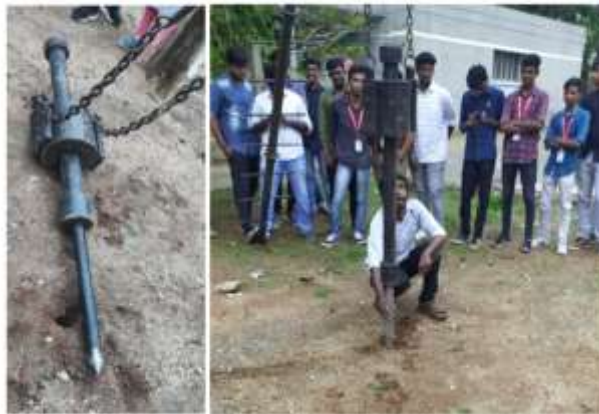
h) Dynamic cone penetrometer i) Demonstration of Dynamic Cone Penetration Test
