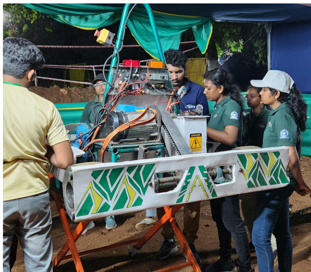
Electrical propulsion system of an Electric go-kart using a 6 kW PMSM motor
